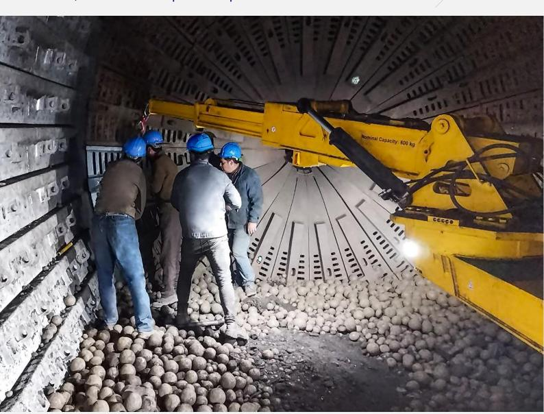
PSDF Co. has designed and manufactured 4, 7, and 8 axes liner handler machines based on its customer's orders. Designing & manufacturing of a customised liner handler machine and its accessories are performed according to your needs. Presented dimensions and technical specifications could be modified in accordance with your requirements.
